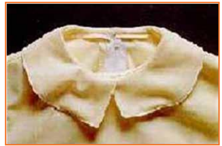
Fig.3.1.22(c): Interlining shrinking
