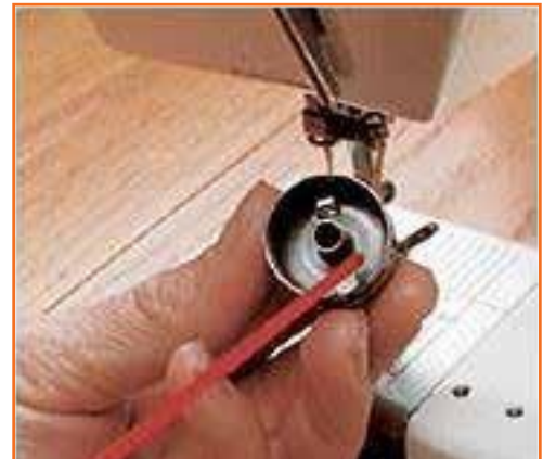
Fig.4.1.2: Cleaning the bobbin and case
