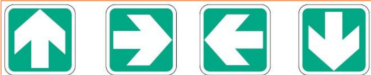
Fig.5.1.17: Signs for emergency exits
