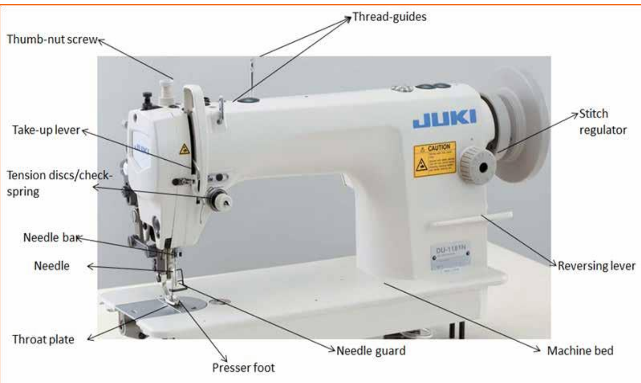
Fig.2.1.20: Parts of a Sewing Machine
