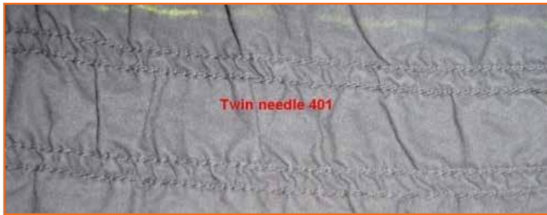
Fig.3.1.9: : Shrinkage pucker occurs during the
