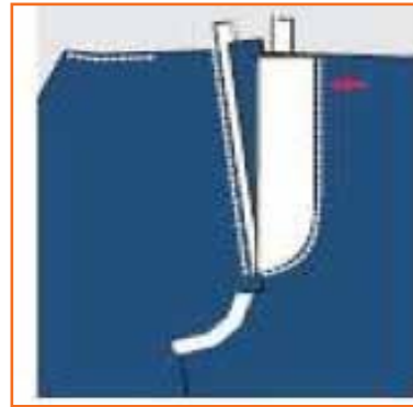
Step 15: Put lockstitch along the ready pattern starting from top to the bottom.
